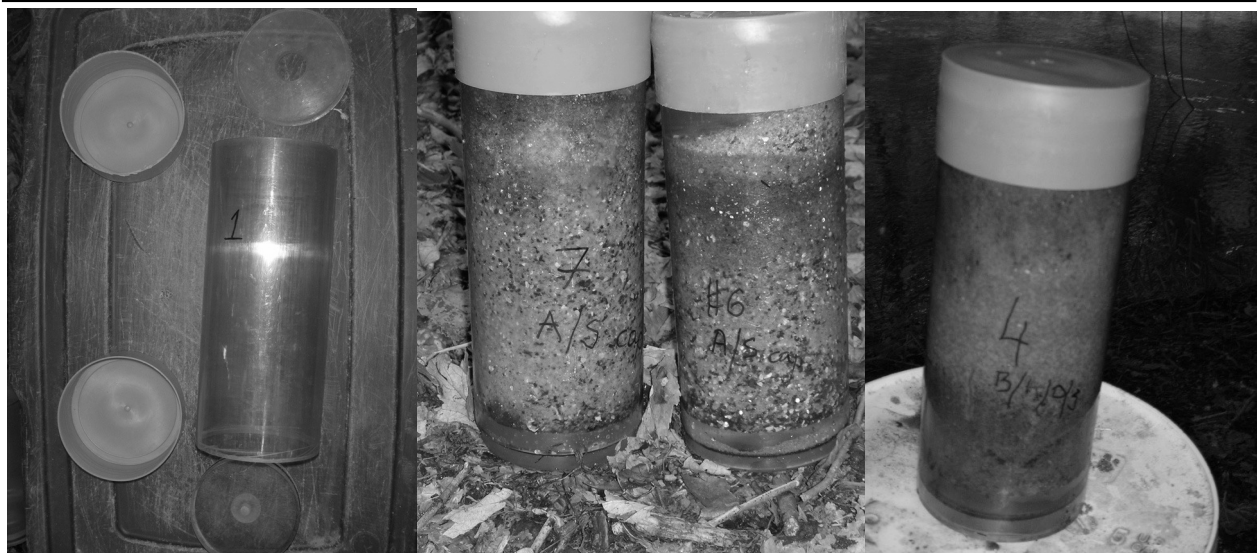
Figure 2. The coring tubes and sediment cores used for evaluation of erosion resistance by an ASSET flume.
