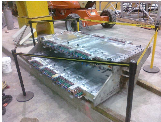
Figure 4. Saskatchewan Accelerator Laboratory pair spectrometer dipole to be used as a spectrometer in the Bethe-Heitler measurement.
