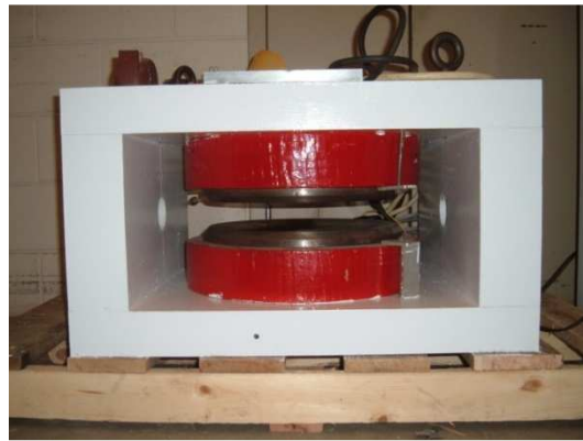
Figure 4. Saskatchewan Accelerator Laboratory pair spectrometer dipole to be used as a spectrometer in the Bethe-Heitler measurement.
