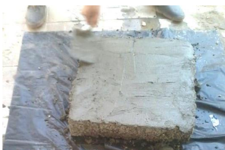
Figure 2: Slab Specimen Mortaring
