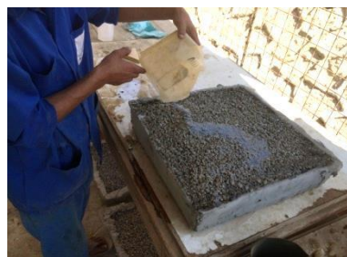
Figure 3: Pouring Polyester for Slab Specimen
