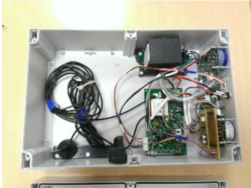
Figure 2: ekoNET device with low-cost electrochemical gas sensors
