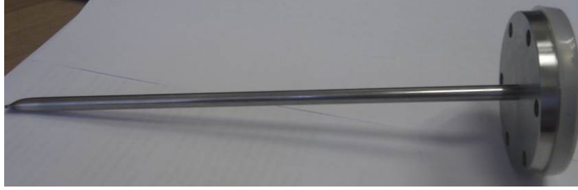
Fig. 2 – ChS-68 membrane arc-welded in a flange
