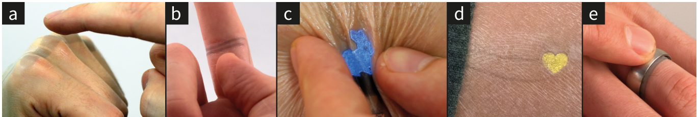
Figure 1: SkinMarks are conformal on-skin sensors and displays. They enable interaction on five types of body landmarks: (a) skeletal landmarks, (b) skin microstructures, (c) elastic landmarks, (d) visual skin landmarks, and (e) accessories.
