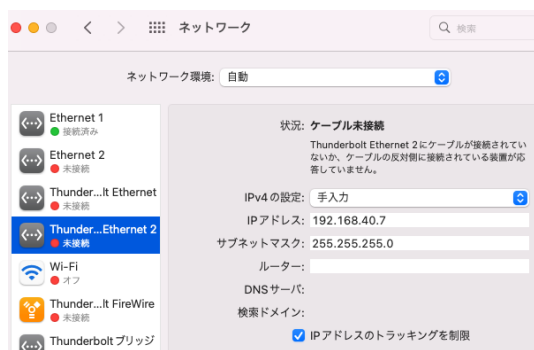
Figure 2: Setting IP addresses with Network panel in System Preferences of macOS.
