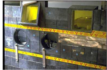
Another view of the Pb shielding surrounding a laminar flow cabinet.
