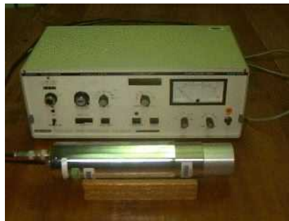
A single channel analyser with a crystal-PMT assembly.
