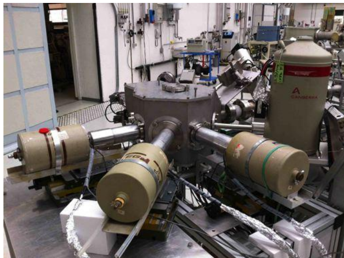
Fig. 2.11. The three HPGe detectors coupled to the multipurpose scattering chamber on the +30° beam line, placed at angles of 0°, 45° and 90° with respect to the incoming beam direction; the two PIXE detectors, a Si(Li) and a SDD are visible as well.
