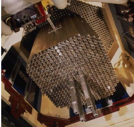
MASURCA - a fast reactor mockup of 5 kW (Cadarache), presently under refurbishment
