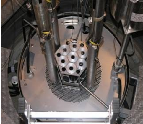
MASURCA - a fast reactor mockup of 5 kW (Cadarache), presently under refurbishment
