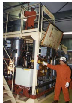
Fig 1: Trainees operating on a real sodium fire exercise and on the filling of a sodium loop
