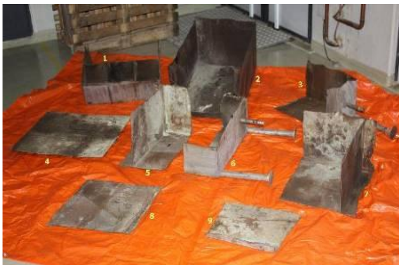
Figure 1 Items carrying radioactive contamination that triggered a radiation alarm at a scrap metal recycling facility. The items were singled out and subject to initial measurement by the competent national authority. Samples were taken to ITU for further analysis.
