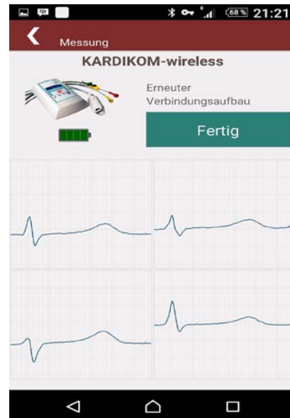
Figure 5: Screenshot of the MedM app with the bluetooth ECG (4 channels) livestream from the Cor/log® BAN BT vital sign data logger.
