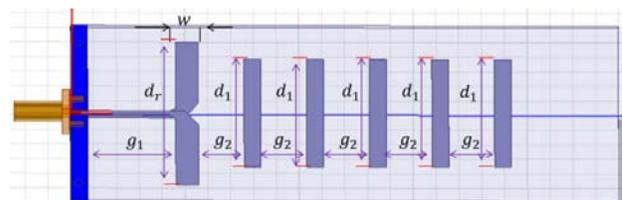
Fig 1. Yagi antenna
