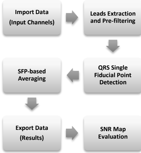
Figure 5. Process diagram for ECG signal analysis and SNR map evaluation
