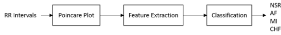
Figure 1. Block diagram of proposed algorithm for classification of NSR and three arrhythmia. (NSR: normal sinus rhythm, AF: atrial fibrillation, MI: acute myocardial infarction, CHF: congestive heart failure)
