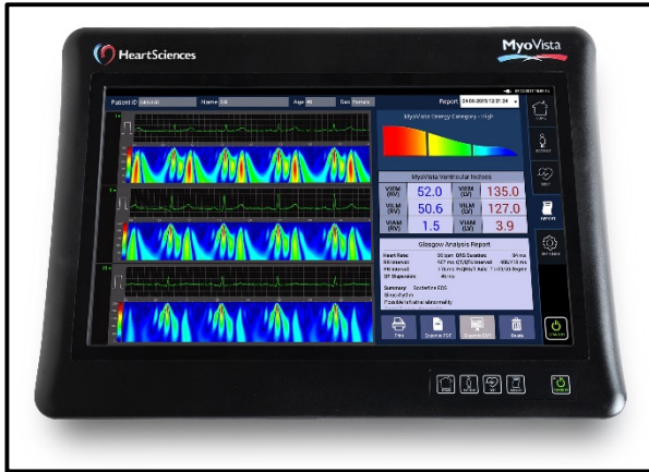
Figure 1: MyoVista Display, (from HeartSciences 2018). The hsECG machine displaying the conventional ECG tracing and the MyoVista energy waveform on the left. On the right of the display is the MyoVista Energy Category (top), MyoVista Ventricular Indices (middle) and University of Glasgow Analysis Report (bottom).
