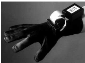
Illustration 18: The 5DT data glove measures finger flexure (one sensor per finger) and the orientation (pitch and roll) of the user's hand. It can emulate a mouse as well as a baseless joystick
