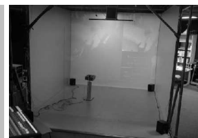
Illustration 15: Through the provision of room-size displays, CAVEs allows for the co-presence of groups, even though all perspective is calculated from the point of view of a single (tracked) user.
