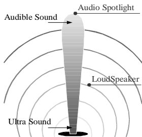
Drawing 2: The ultrasound, which contains frequencies far outside our range of hearing, is completely inaudible. But as the ultrasonic beam travels through the air, the inherent properties of the air causes the ultrasound to distort (change shape) in a predictable way. This distortion gives rise to frequency components in the audible bandwidth, which can be accurately predicted, and therefore precisely controlled.
