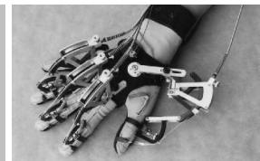
Illustration 20: The cyber-grasp uses an exoskeleton to provide haptic feedback.
