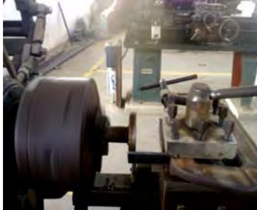
Fig.1. Experimental set up for making low frequency cyclic load.
