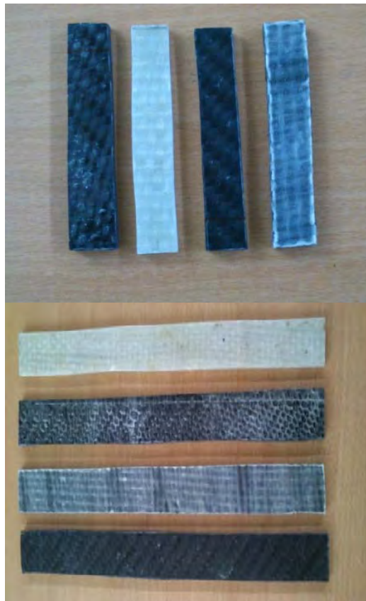
Fig.2. ASTM Standard Specimen prepared for Flexural studies (Top) and Tensile Studies (Bottom).
