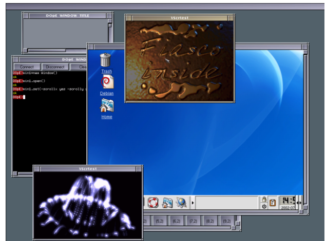
Figure 10: Screenshot of DOpE running two real-time client applications and L4Linux
