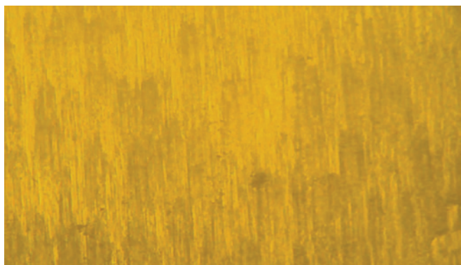
Figure 12 (b): Etch pattern of CN single crystal (etching time 10 s).
