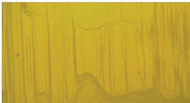
Figure 12 (a): Etch pattern of CN single crystal (etching time 5 s).
