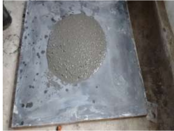
Fig. 1 Slump Spread for SCC with M-Sand
