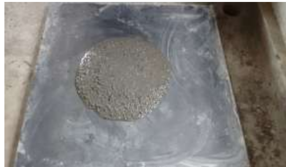
Fig.2 Slump Spread for SCC with WCR
