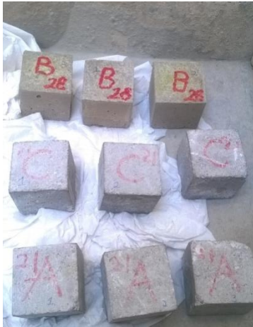
Fig. 12. Mortar specimen (B) in distilled water and mortar specimen (A and C) in sulphate solution
