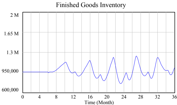
Figure 2: Finished Goods Inventory Oscillations Due to 10% Increase in Demand at Time = 6
