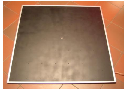
Fig. 2: Plane testfield with active lamps
