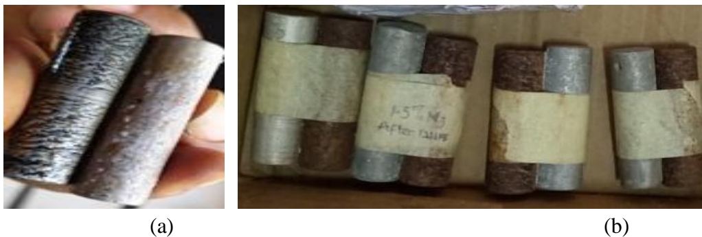
Figures 6: (a) Sample of the specimen before post immersion cleaning (b) Samples of the specimens after the corrosion test (gravimetric technique)
