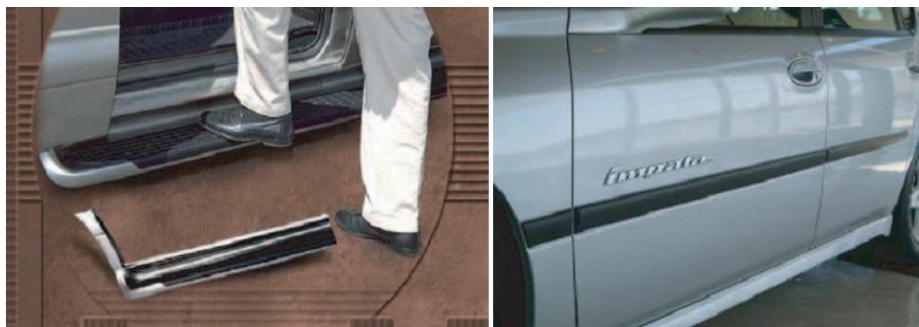
Figure 8: M-Van step Assist: 1 st commercial launch for TPO nano-composite application [66]
