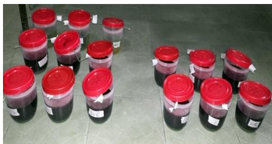
Fig. 11. Coupons in Corrosive Media (Distilled Water)
