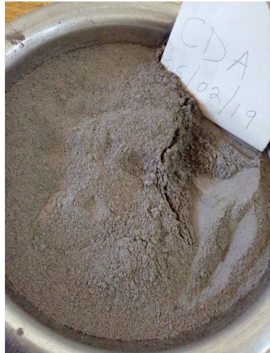
Fig. 1: The texture of cow sludge ash passing through 150 µm sieve
