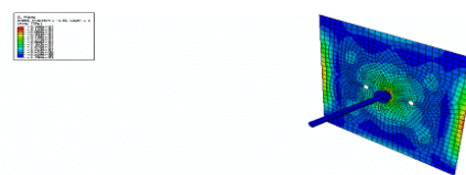
Figure (5) Stress contour for composite plate with one hole of diameter (10) mm at (CCCC) boundary condition.
