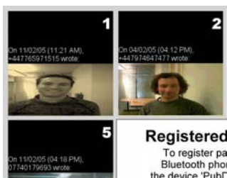
Figure 8: Annotating the presentation with digits to enable a user to select a vCard for transfer.
