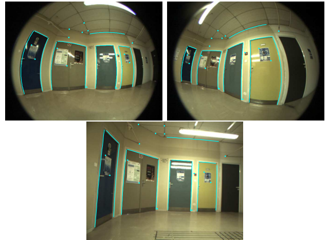
Figure 3. Fish-eye and perspective images with point and line correspondences
