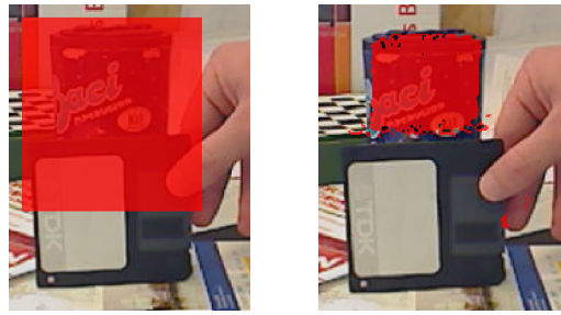
Figure 5. Effect of depth filtering to avoid the influence of background and occluding pixels in histogram computation. Left, in red: full candidate region. Right: filtered region using depth dissimilarity.
