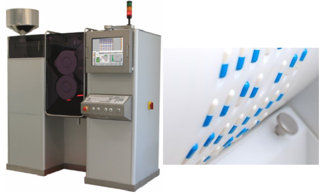
Figure 4. Sensus SPINE visual quality inspection machine (left), which automatically inspects and sorts pharmaceutical capsules or tablets (right); the speed for capsules is up to 180,000 capsules per hour.
