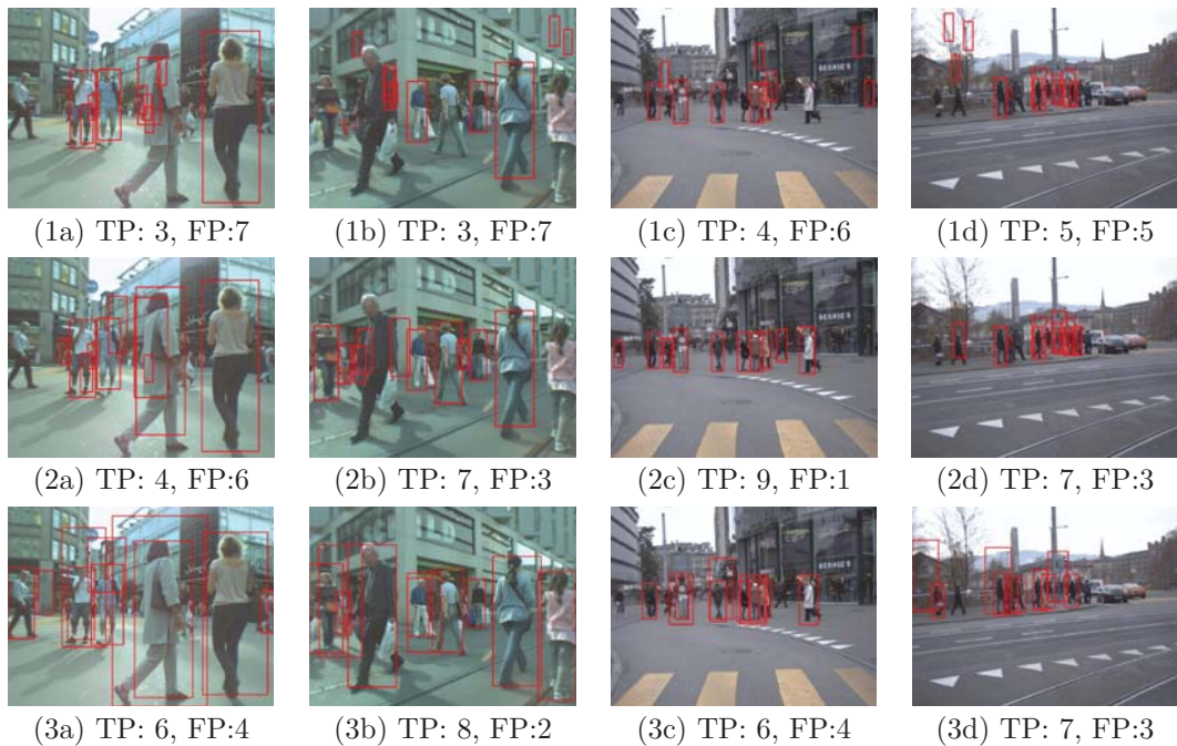
Figure 3. Some results of the three systems. The three rows correspond to the results from the baseline detector, our method and UoCTTI detector respectively. (TP: true positive, FP: false positive.)
