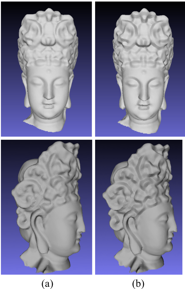
Figure 5. Result: (a) 3D shape of the plaster statue profile before sharpening. (b) 3D shape of the plaster statue profile after sharpening.
