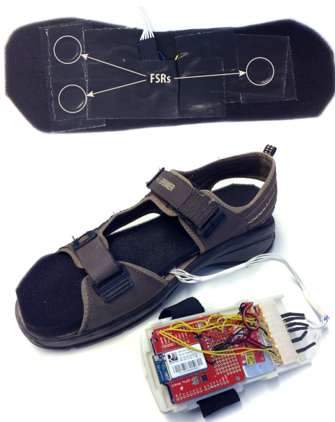
Figure 2: The sensor sole with three force sensitive resistors attached with duct tape (top) and a sandal connected to the GPSP interface with exposed electronics (bottom).
