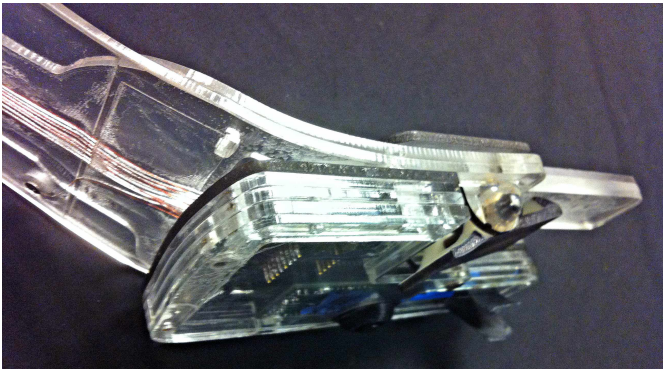
Figure 4: Detail showing the laminate construction of the Ribs, with the protrusion and clip for mounting visible on the right.
