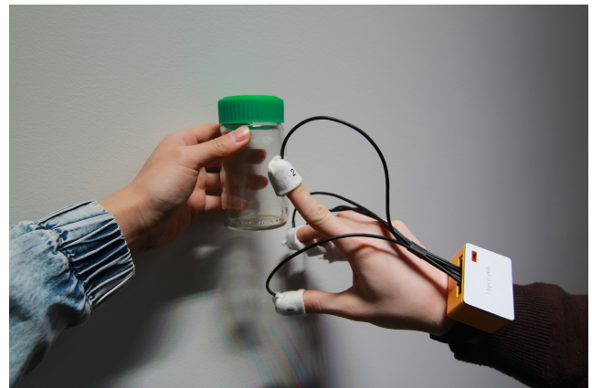
Figure 1: The FingerSynth enables its wearer to play music anywhere while exploring the resonant qualities of objects around them.
