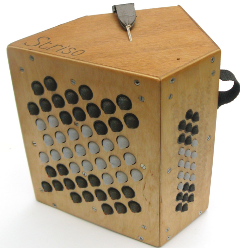
Figure 1: The Striso, with for the right hand the DCompose note layout and for the left hand a reduced size note layout for accompaniment.
