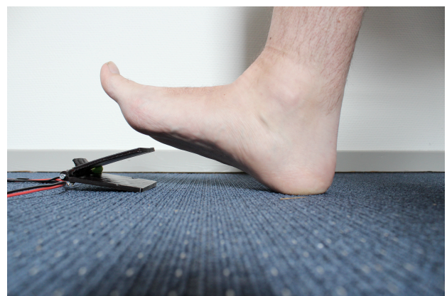
Figure 9: The 3D printed foot pedal used to activate the actuator strumming the strings of the guitar. The print is fitted with a momentary button that is connected through wires to the Arduino inside the guitar.
