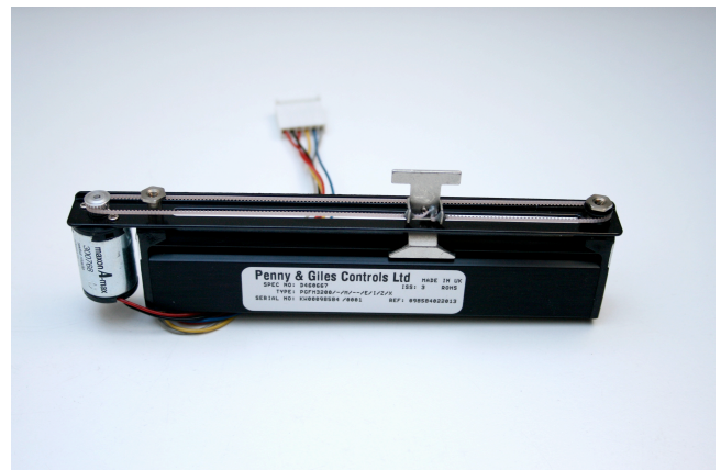
Figure 2: Motorized fader used as the actuator for driving the pick back and forth over the strings of the guitar.
