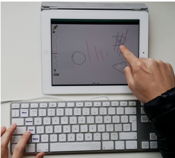
Figure 2: The user interface for Drawchestra comprises an iPad and a keyboard. The iPad is employed as a slave touch screen through which user can draw and manipulate shapes. The keyboard, which is labelled for the convenience of the participants, is used to switch between the modes of user interaction due to the current system does not support multi-touch.
