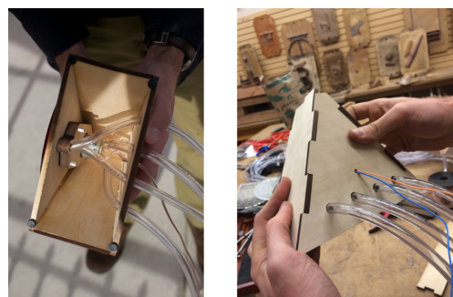
Figure 8: The inside and back of the siren disk stand.
