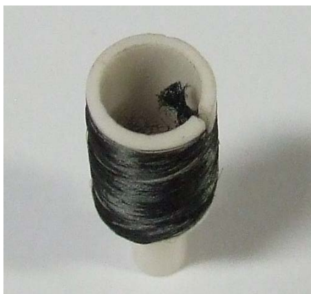
Figure 2. Fixed fiber sample on alumina cylinder after thermal treatment.
