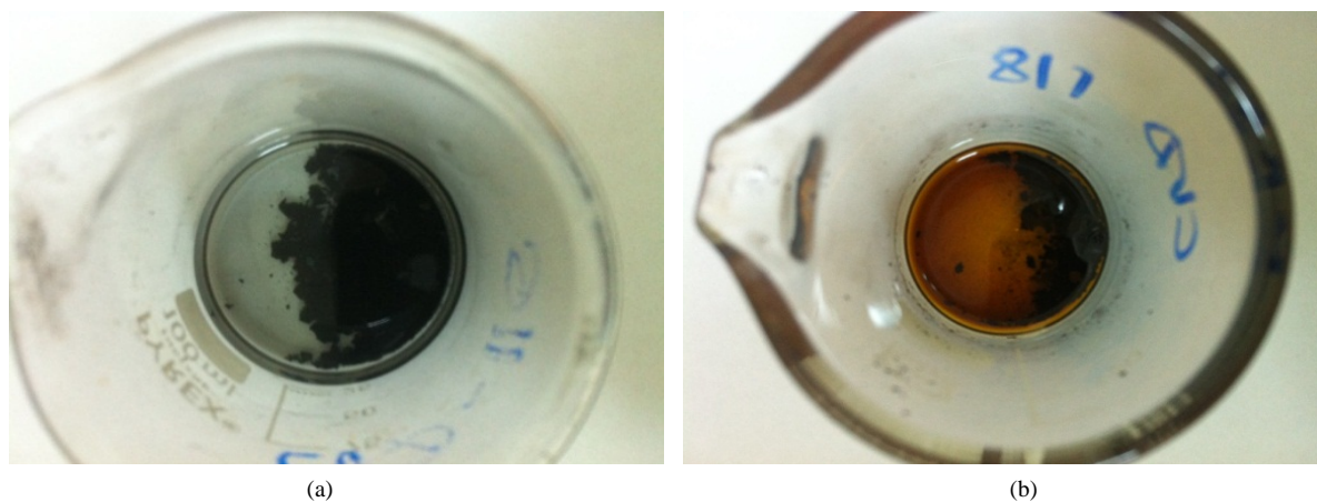
Figure 3. Washing of CNTs with: (a) cyclohexane; (b) toluene.
