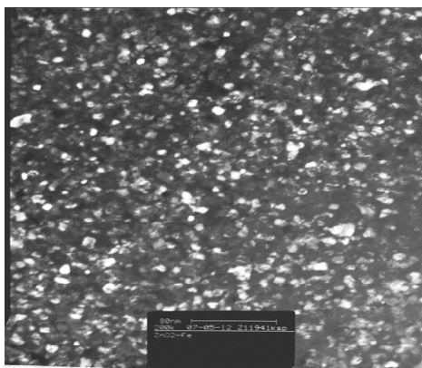
Figure 7. The dark field TEM image of nanocrystalline ZnO.
