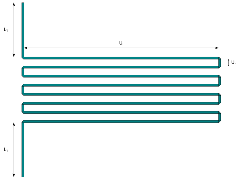
Figure 6. Simplified folded microstrip delay-line.
