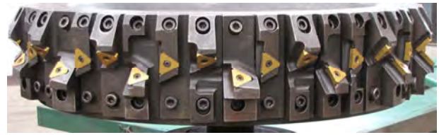
Figure 4. Plate edge milling cutter with 40^\circ , 48 numbers cartridges.
