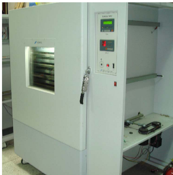
Figure 1. Shaking apparatus for testing with fuel types and specimens.
