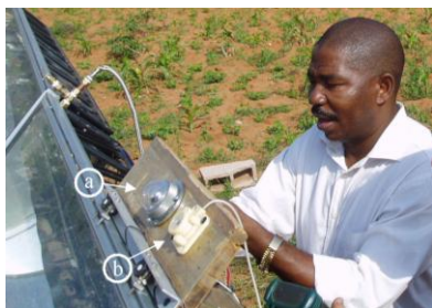
Figure 2. Two of the installed pyranometers: a) CMP11 LU and b) new SRS1000
